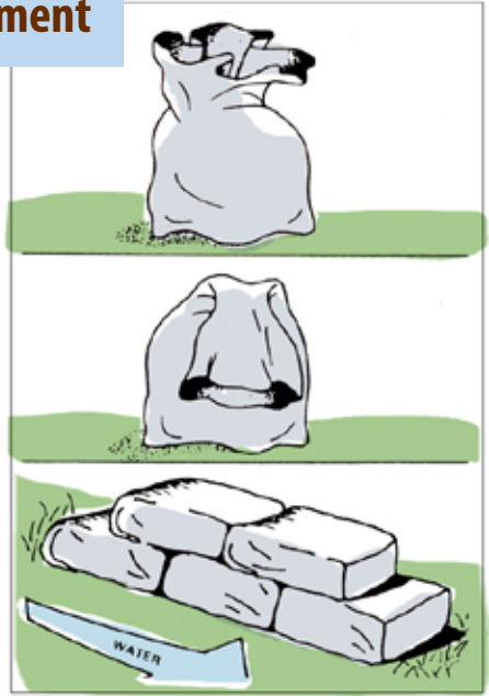
Figure 9: Sandbag Filling and Placement – Proper filling and placement of sandbags is important.
