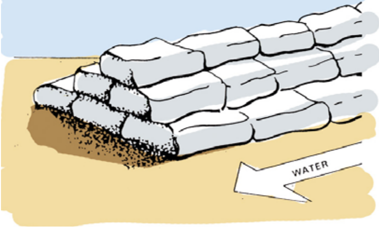
Figure 11: Sandbag Stacking – Allow for a wider sand bag wall when stacking sand bags higher.
